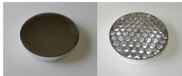
Fig. 12. The fabricated 175-mm spherical magnesium-alloy mirror. The left and the right panels show the mirror surface and backside of the mirror, respectively.
