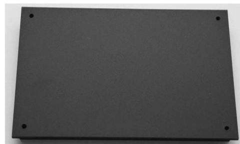
Fig. 2. Morphology of micro-arc oxidation coatings with thermal control of magnesium alloys [110].
